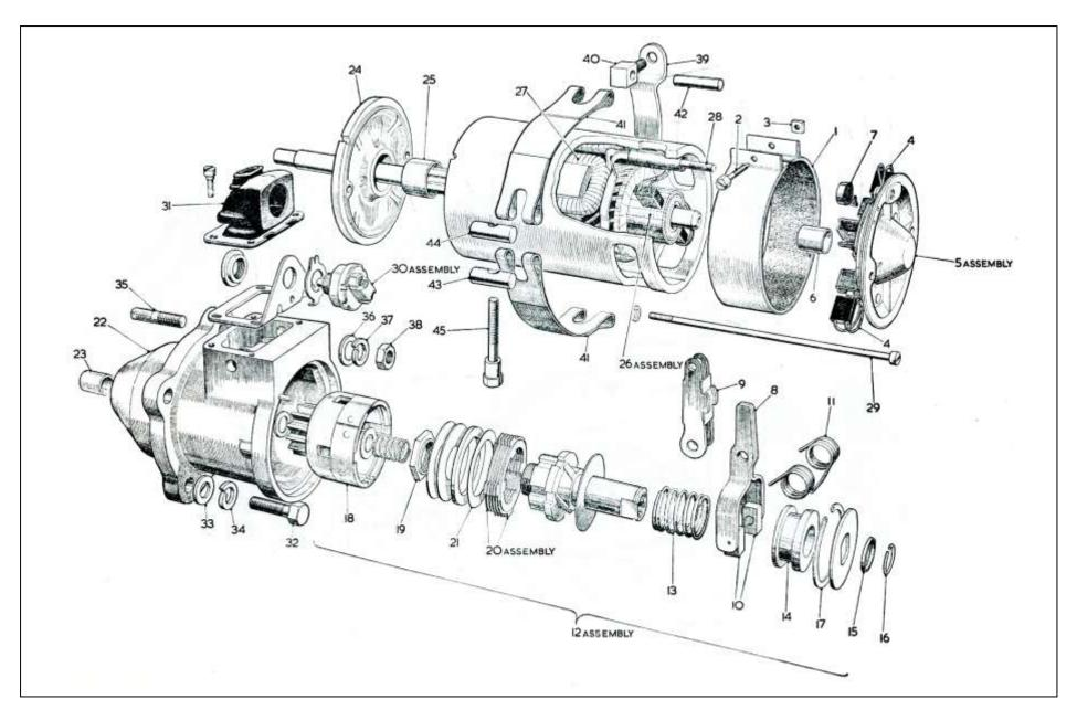
Exploded view drawing of the Lever type Starter Motor. Part number AMK1335.
