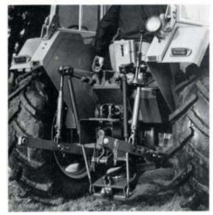
Simple control from a lever easily operated from the driver's seat, combined with the ability to see the coupling operation, cuts turn-around time to a minimum
