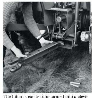
drawbar by removing two pins, withdrawing the bar and turning around. When reinserted, the bar can be pinned and used in the short or extended position. Although preferable to use the hook, there are occasions when the clevis must be used. It is possible to remove one leg of the clevis and swivel ball joint is incorportated to protect
