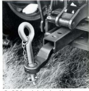
For P.T.O. work the hook and bar is extended so that the point of towing is 14 inches (355 mm) to the rear of the P.T.O shaft. One central and two offset positions can be used to cover the full range of P.T.O. work.
